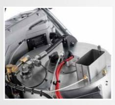
**OPTICAL FLAME MONITORING** AND THERMAL OVERLOAD PROTECTION Electronic monitoring of combustion: Kränzle therm devices have a photocell to monitor the burner flame. This ensures safe operation at all times, even if the user is not near. Additionly, an overheating protection sensor measures the temperature at the exhaust; switching off heating automatically if more than 260°C is detected.
