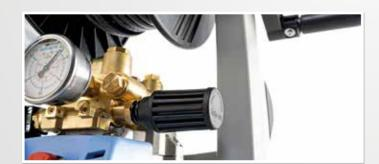
**PRESSURE REGULATION | STAINLESS STEEL PRESSURE GAUGE** With all high-pressure cleaners (except the K1050-series), the working pressure and water quantity can be individually adjusted to the respective application. The large stainless steel pressure gauge provides a clear reading of the set working pressure. It contains a glycerine liquid that dampens possible fluctuations of the pointer.
