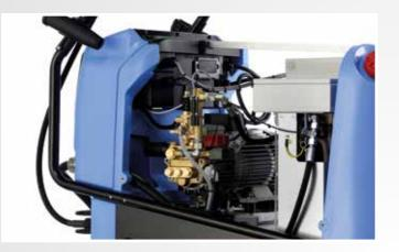
**ELECTRICALLY HEATED INSTANTANEOUS WATER HEATER** Stable heat: the instantaneous water heater can be operated with up to 48 KW and enables even in continuous operation Temperatures up to 80 °C. It ensures a uniform water temperature and is therefore ideally suited for cleaning of fats and oils.
