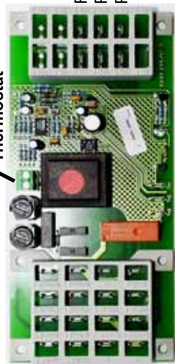
Flow controller Pressure switch Burner release Pressure switch Motor Start/Stop
