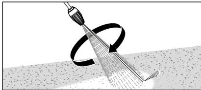
12. When using the filth killer lance make sure that lance points downward when starting.
