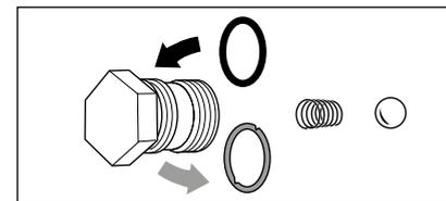
If sealing rings are defective replace O-rings at once.
