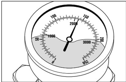
Having closed the trigger gun with safety catch, the high-pressure cleaner must shut down and the stainless steel pressure gauge must show „0“ bar. If not shut down and the stainless steel pressure gauge continuously shows full pressure, this could be due to leakage at the high-pressure pump, at the pressure switch, at the high-pressure hose or at the trigger gun with safety catch.
