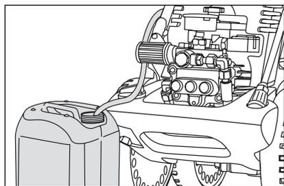
1. Place chemicals filter into container with additives
