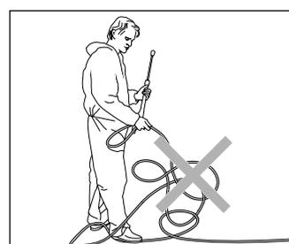
Never pull the high-pressure hose if it has formed kinks or "nooses"! Never pull the high-pressure hose over sharp edges!
