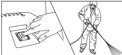
11. Switch on high-pressure cleaner with opened safety trigger gun. Bleeding of the high-pressure cleaner: Pull and release trigger of safety trigger gun several times. Start cleaning task.
