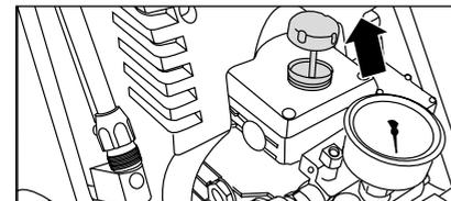
9. **Each time check oil level at the oil dipstick prior to putting the high pressure cleaner into operation.**
