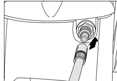
8. Connect water hose to water inlet (minimum requirements; 5 m hose length, cross-section  $\frac{3}{4}$ ", 10 bar). The high-pressure cleaner may be connected to a water mains (1-10 bar pre-pressure) with either cold or hot water (up to 60 °C). The medium quadro series provides the opportunity of sucking in water out of a container (see direct suction).
