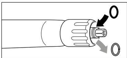
Switch off the cleaner. Shortly press the trigger of the trigger gun with safety catch to decrease the pressure. Remove high-pressure hose, trigger gun with safety catch and lance and check the O-rings. If the O-rings are damaged they have to be replaced.
