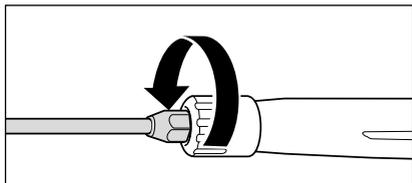
6. Screw together lance and safety trigger gun pressure tightly.
